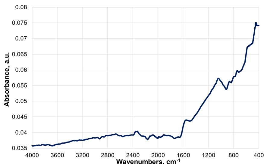
Figure 5. FTIR spectrum of biochar (final product)
