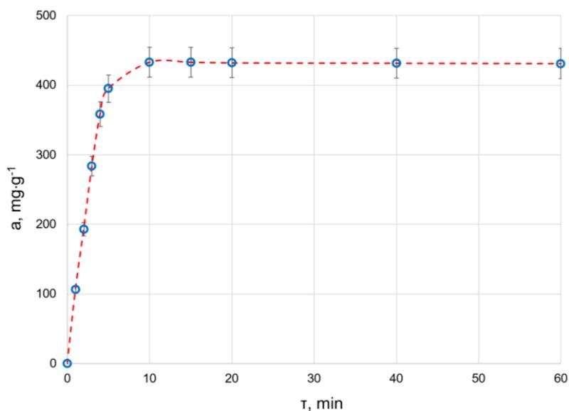
Figure 6. Adsorption kinetic curve of ibuprofen onto biochar
