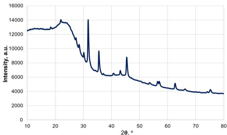
Figure 4. XRD spectrum of biochar (final product)
