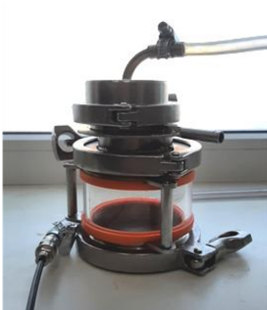
Figure S1. Image of the vacuum filtration device
