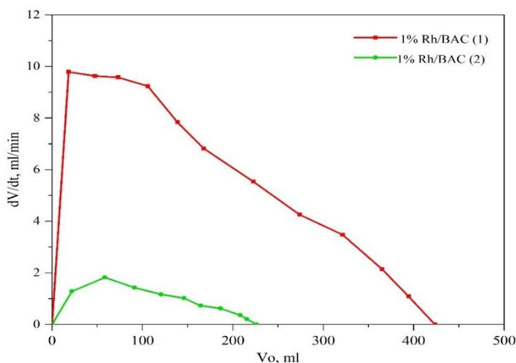
Figure 5. Kinetic curve of benzene hydrogenation with 1 % Rh/BAC.
