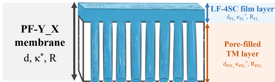
Figure 6. Schematic illustration of the PF-Y_X sample, consisting of a layer of LF-4SC ion-conducting material and a track membrane with straight pores filled with the same ion-conducting material
